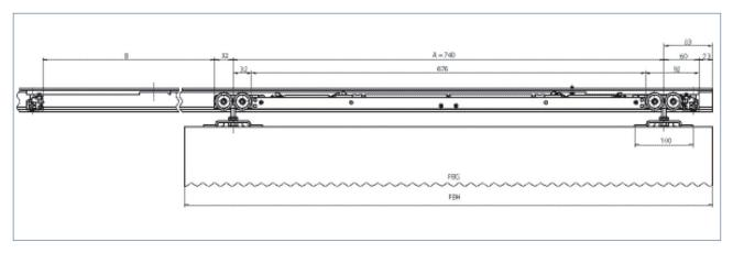
FBG= Glass leaf width FBH= Wood leaf width A = Suspension bolt spacing
